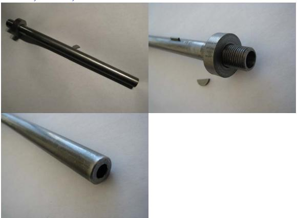
Specs: The steel headstock spindle (length approximately 7.5" - most pieces are a little longer, O.D.  $\frac{1}{2}$ " regular stock) has a standard ANSI Morse #0 arbor and  $\frac{1}{2}$ "-20 TPI threads (thread length 0.55"). A round collar hold by a set screw #10-32 is included. The spindle is drilled through 0.25". All dimensions are approximate. The piece has a slot for a Woodruff #1 key (key included) at 2.614" from the front end of the spindle.
