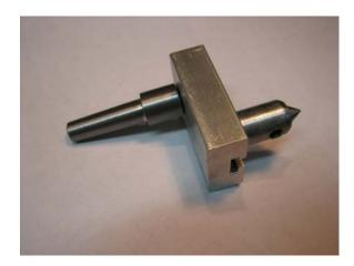
**Procedure:** Extend the tailstock spindle by about ¼". For best fit, *slightly* (and carefully) slam the taper in the spindle *by hand*. To remove the taper, pull back the spindle. Typically, taper arbors/spindles have an internal draw bar, which will push out the taper.
