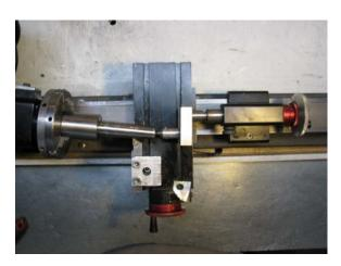
**Typical application:** Accessory for benchtop / tabletop lathes. Adapter mounts in a Morse #0 arbor, e.g., in the tailstock spindle of a small tabletop lathe and connects to a dead center (pin).
