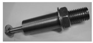
Procedure (1"-8) Screw the 1"-8 adapter over the ¾"-16 end of the spindle. A slot is milled in the front end of the 1"-8 spindle, a key stock is included. Don't use plier to tighten or untighten the threads which would damage the threads. Place some cutting oil on the threads. Tighten first the 1"-8 adapter then the spindle. Important, when mounting the chuck then use either the provided washer or a 1"-8 nut which will act as a shoulder for the chuck.
