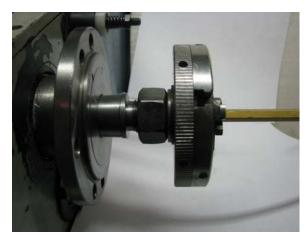
Procedure (3/4"-16)-short chuck For smaller and shorter chucks use the ¾"-16 spindle, but screw a ¾"16 nut first over the threaded end of the spindle. You may use a washer. Tighten the chuck against the nut/washer using a wrench. Hold nut with wrench and screw lathe chuck against the nut which will act as a shoulder. You may want to use a washer.
